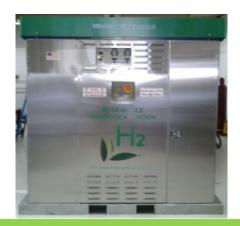
Palletized, 4 kilogram per day production, Scalable Hydrogen Fueling Appliance With 8 kilograms storage at 6,000 psi with fixed orifice fueling and J2600 nozzle J2719 fuel quality
